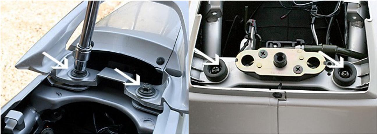
**Step 6:** Undo the two screws next to the battery.
