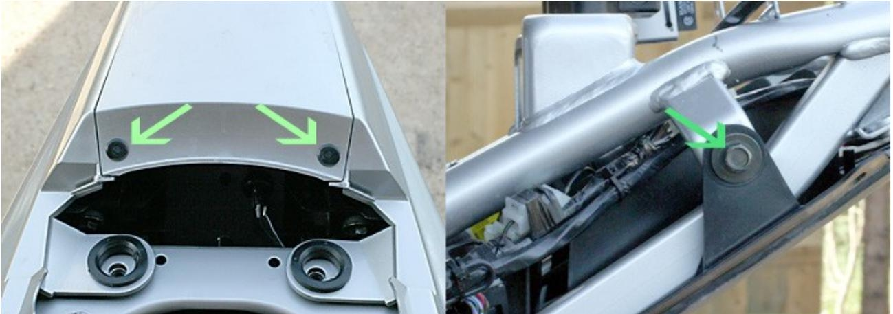
**Step 14:** And remove the two bolts at the front that may be hiding under your wiring loom.
