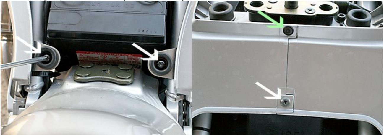
**Step 8:** Remove the four pop fasteners underneath the seat tail cover.
