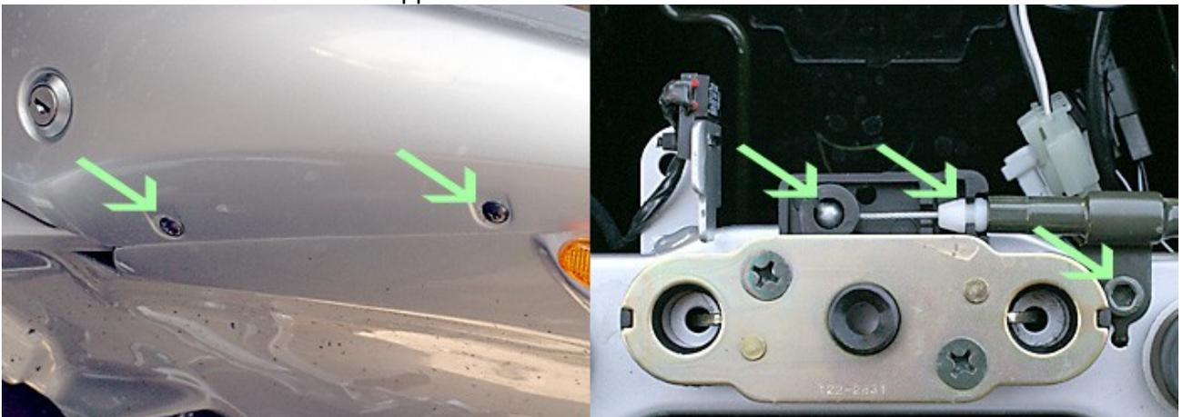
**Step 10:** Although not really necessary you can undo the two pop fasteners illustrated to remove some of the strain for removal.
