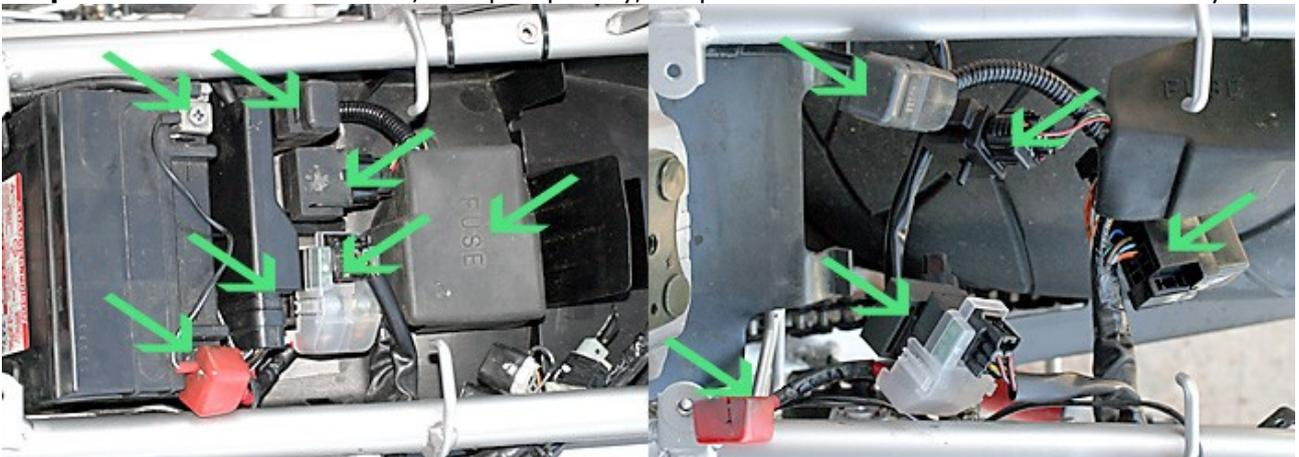
**Step 19:** Unhook the undertray from the four plastic lugs where you removed the bolts, slide it forward and take it off.
